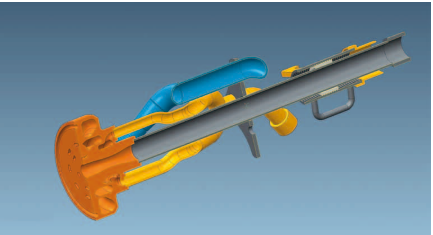
Fig. 6 - SMS latest Conso burner design with head printed with 3D additive manufacturing technology
