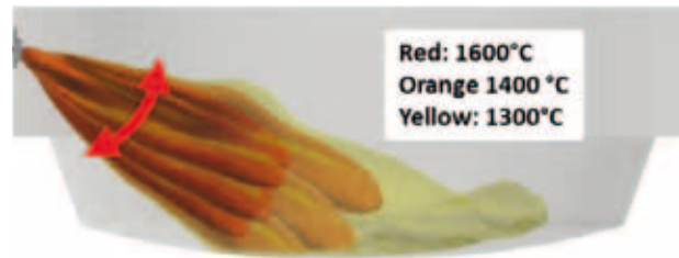
Fig. 17 - Schematically moving volume of the burner during meltdown
