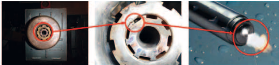
Fig. 20 - Electrical ignition of the gas by sparking
