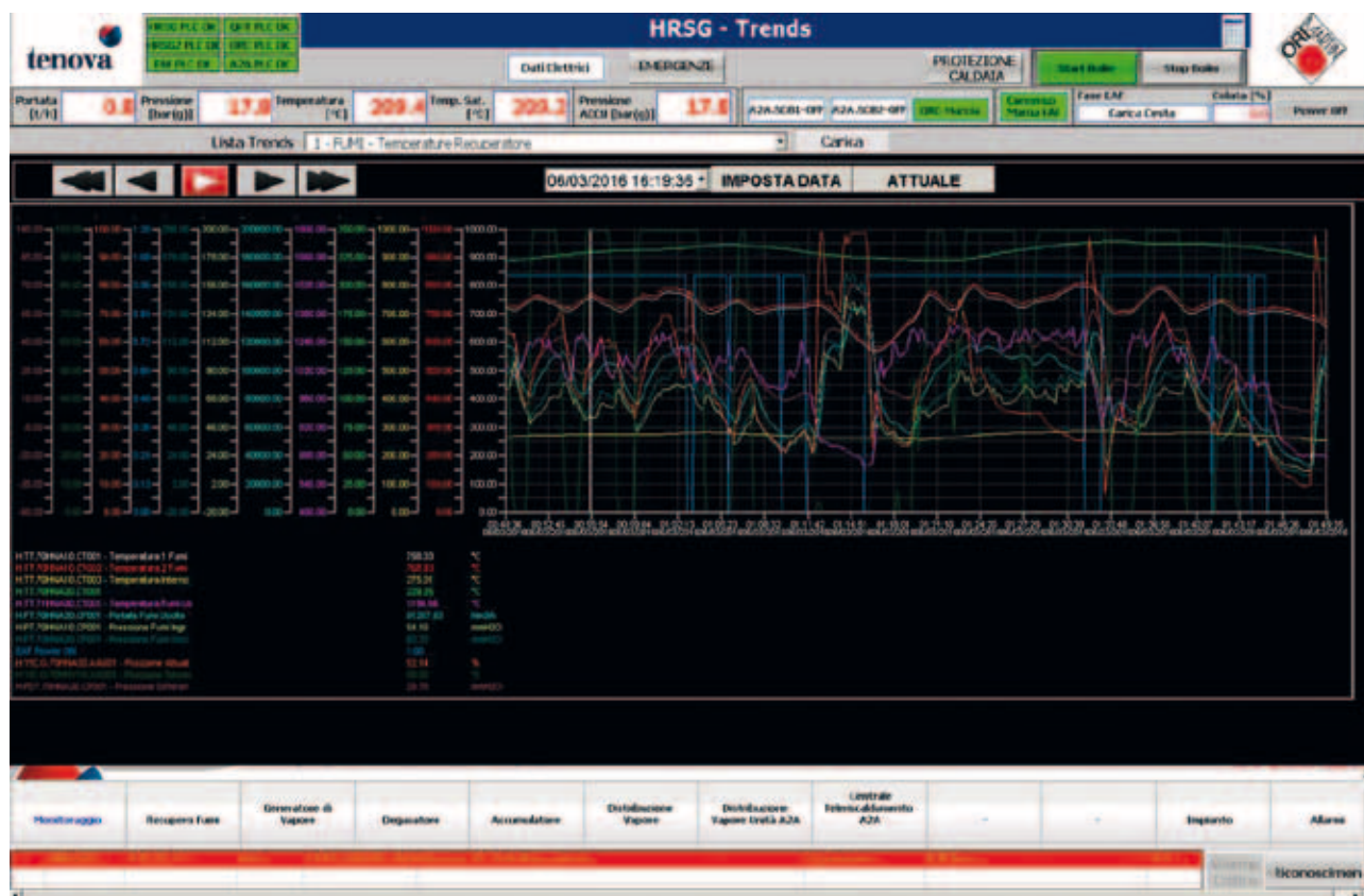
Fig. 10 - The new iRecovery system in operation, off-gas temperature cycle in a sequence of representative heats.
