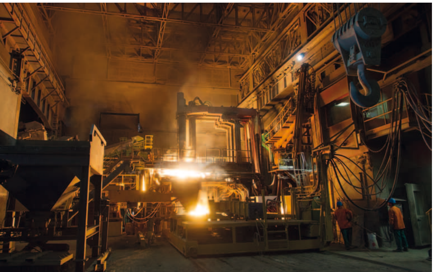
Fig. 1 - The new revamped Consteel®, connecting car side.
