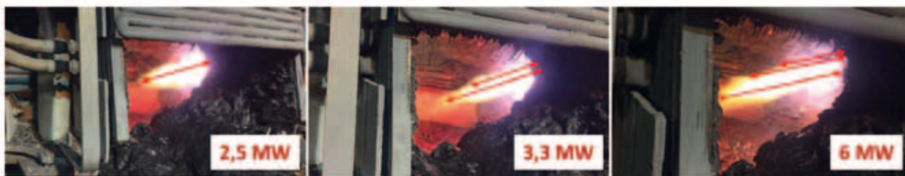
Fig. 10 - Change of the flame length as function of the flame-power and flame prolonging by increasing the power
